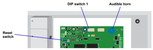
To re-enable the horn, set DIP switch 1, the first switch, to the OFF position (down) and press the reset button.
